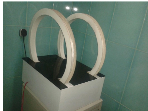
Figure 1. Device used for producing an alternating magnetic field (frequency 50 kHz) for the experimental group
